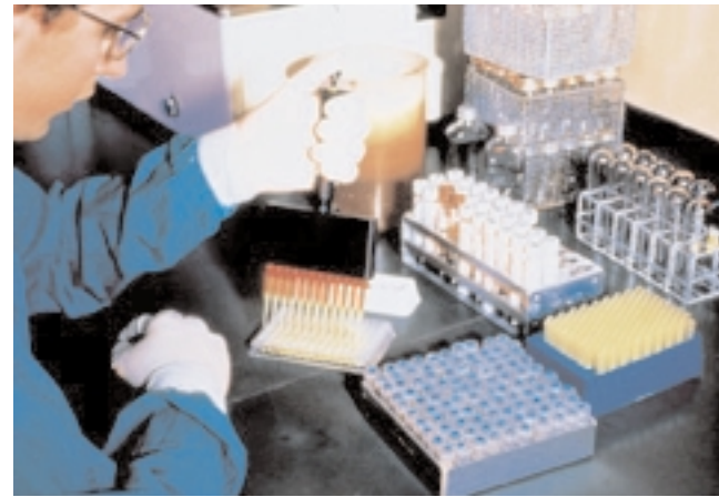
Powder from gloves may fall into lab assays contributing to erroneous results.
